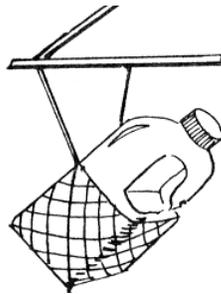
With a plastic net, suspend the bottle from a metal support. Let one piece of plastic hang down to suspend the soap from. If a net is not available, two holes can be made in the back of the bottle, and the Tippy Tap can be suspended by connecting a string through those holes to the support.
