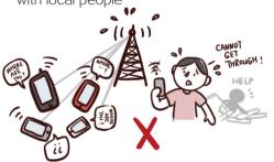
Signals will be transmitted through local base station and the local communication networks will be further burdened
