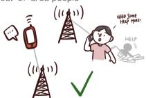
Signals will be transmitted through an out-of-area base station and the local communication networks will NOT be further burdened
