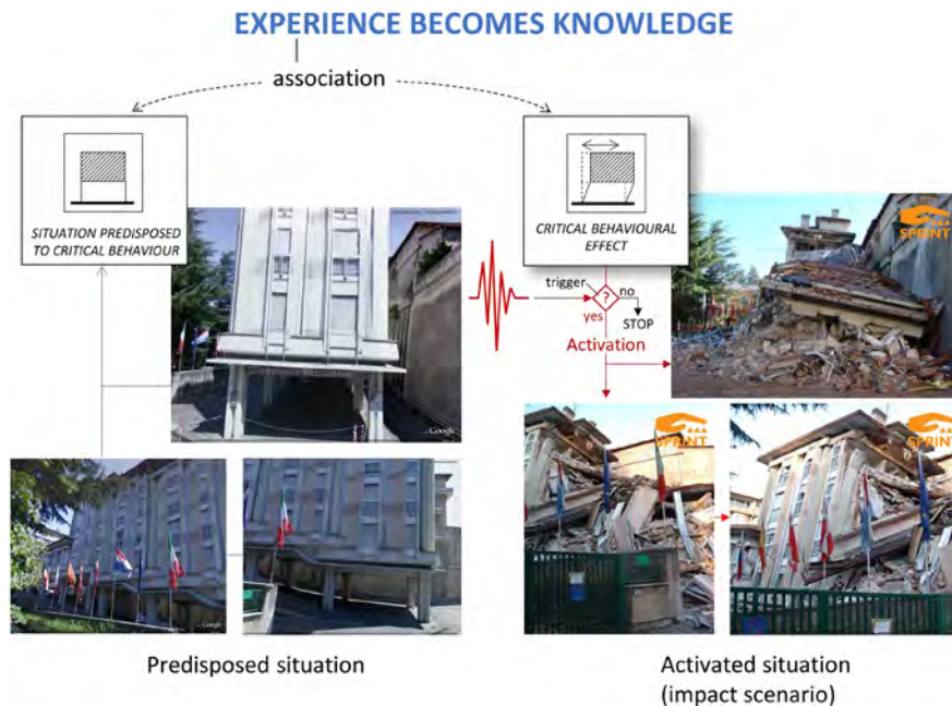
Fig. 1.20 Observation of the damage to facilities after a hazardous event such as an earthquake, shown in the figure, allows experts to associate by a priori evaluation the features of specific critical situations
