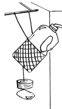
Make a hole in the center of a bar of soap. From the hanging piece of plastic, suspend with a string the soap and a plastic or metal cover (such as a tin can) to protect it from sun and rain.
