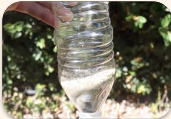
Step 4: fill bottle with sand /charcoal about 2 inches
